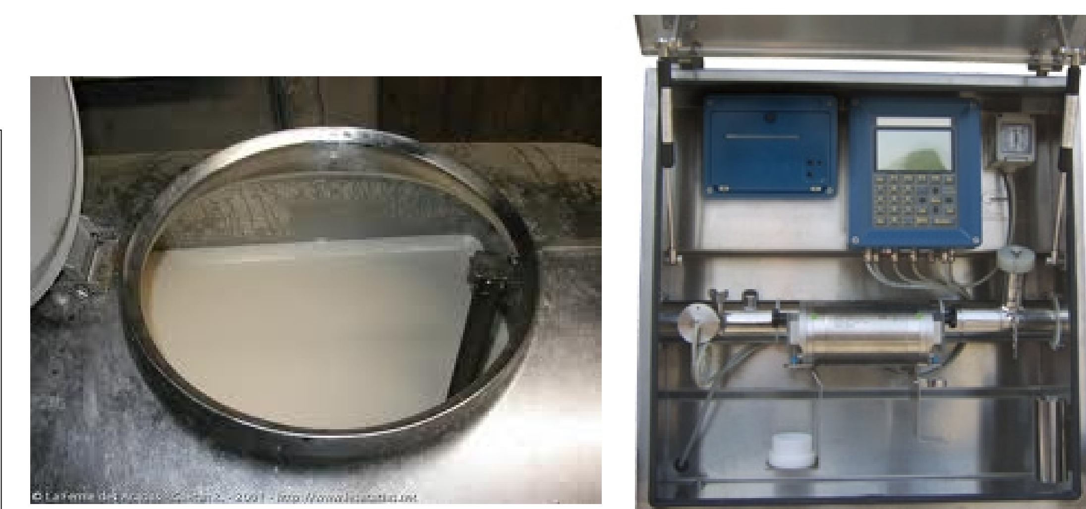
Figure 2. Farm tank with calibrated bar (left) and the automated system (right).
