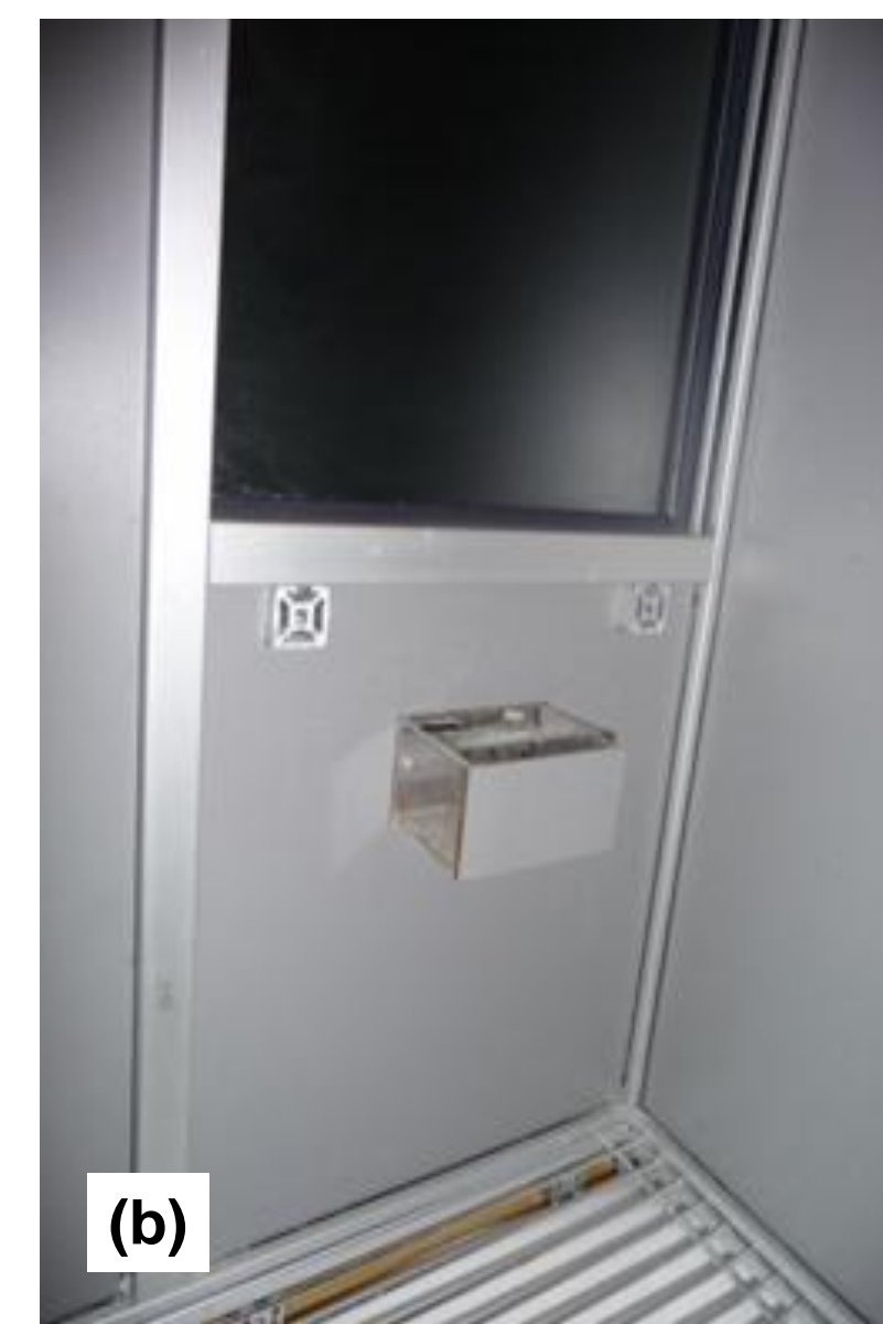
Fig. 1 The operant chamber. (a) outside view; (b) inside view with opened automatic feeder after correct response to positive stimulus; (c) CD-ROM stepper motor controlling feeder
