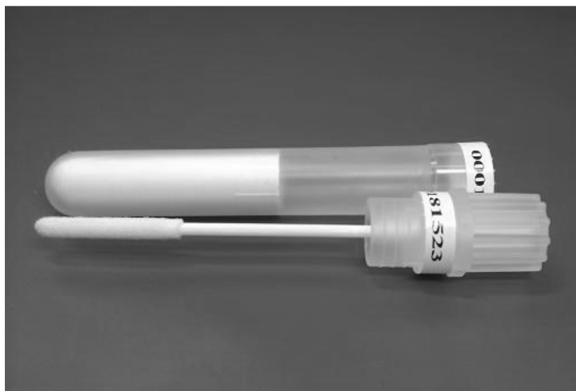
Figure 4: Swab by Prionics [5] used for collecting the DNA sample from an animal. The swab can be ordered through the DNA laboratory, using an ordering form provided by the LAREU system. The swab carries a unique number for proper identification.
