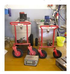
Feed:water = 1 : 2.75 Temperature = 20 °C Fermented until steady state
