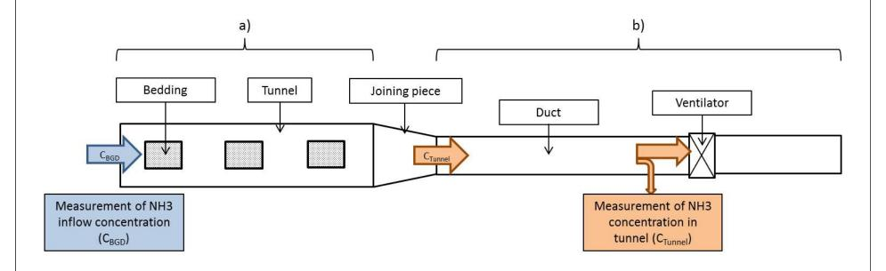
$E_{Bedding} = Q * (C_{Tunnel} - C_{BGD})$
