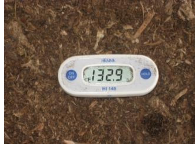
Example of compost heating well with high temperature and dry material.
