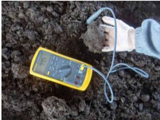
Example of compost that is too wet with insufficient temperature.
