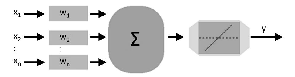
The aggregation function processes input data and weights into the argument of the activation function
