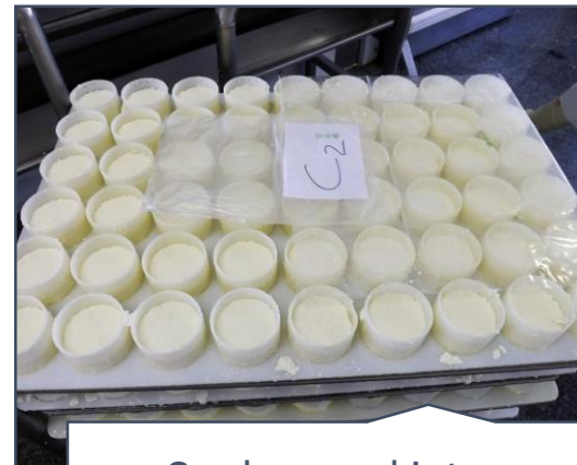
Curd poured into cylindrical multi-moulds
