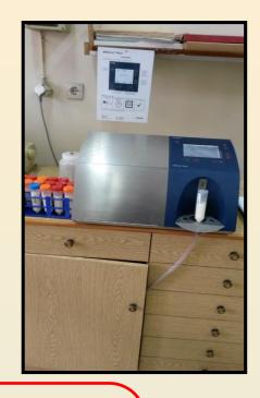
Colostrum total solids determination using a digital BRIX refractometer
