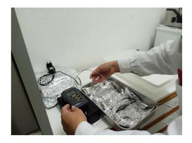
Samples placed in a conventional oven and cooked until reaching the temperature of 80°C in their thermal centre.
