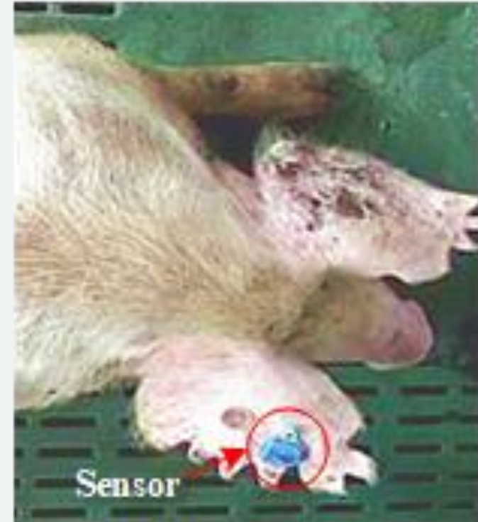
Fig. 4. An acceleration sensor is attached to the RFID ear-tag on a sow.
