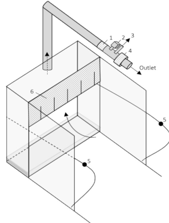
1: Flowmeter, 2: T-RV sensor, 3: Sampling point, 4: Fan, 5: Background sampling points, 6: Rear flap.
