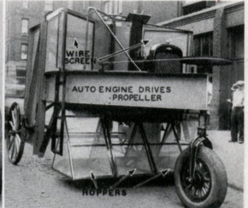
This 'hopper-killing device is the invention of Joseph Dillman, North Dakota farmer, and Henry Olson, of Minneapolis, who are shown at the left above. Note the four suspended wire cages, at right, into which the dead insects are blown and collected.
