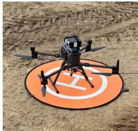
Quadrotor UAV RTK (max payload 2.7 kg)
