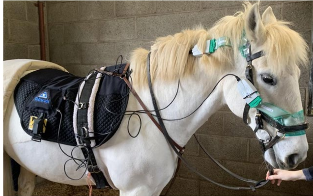
Plate 2: Horse with full Tekscan Pressure Sensing System
