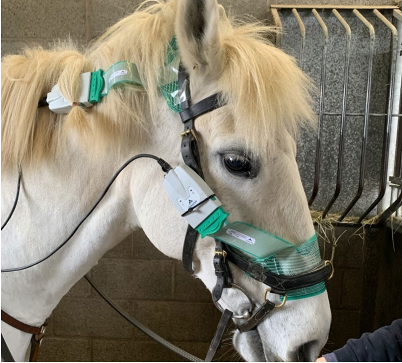
Plate 1: Horse with Tekscan Pressure Sensing System attached.
