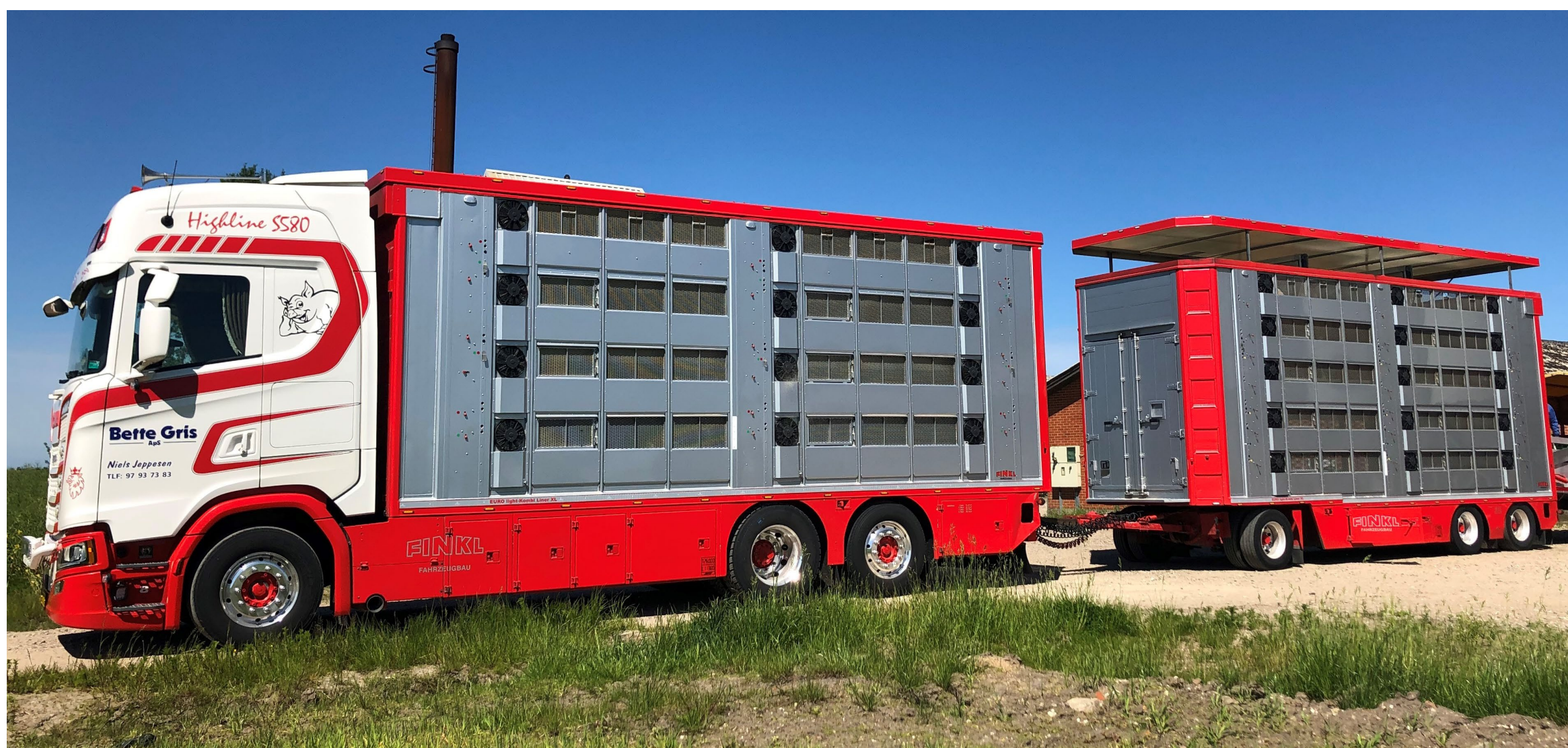
Fig. 1. Photo of the vehicle (4-deck lorry with 5-deck trailer) used for experimental trials. The photo shows a situation during the process of loading pigs onto the trailer with roof lifted, shutters for natural ventilation fully opened and separate shutters in front of the mechanical ventilation fans also pulled down. (Photo: Aarhus University)
