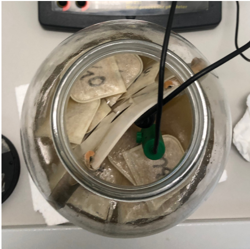
Fig. 4 Daisy II jar with sample bags, ruminal fluid and buffer. pH measurement during fermentation.
